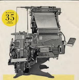
ONE OF THE most versatile of Super Display models, which produces mixed composition in the same line from small body faces through normal 36 point-at straight-matter speed.
